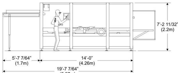
INSTALLED LENGTH BETWEEN CUSTOMER SUPPLIED CONVEYORS
